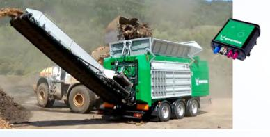
"The hardware has to fulfil the rough environmental and working conditions. This, for example, could mean high temperatures, vibrations or formation of dust. By using the CAN Gateway, a reliable data connection is provided."
